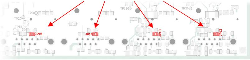
Position of the solder fields on the bottom side of the circuit board for the 5-Volt supply at the D-Sub connector (JP12 on the right, JP15 on the left)
